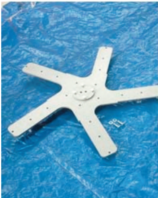
AFTER DISASSEMBLED BLADE SUPPORT, DISASSEMBLY HUB
