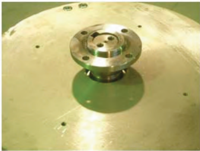
AFTER DISASSEMBLED BLADE SUPPORT, DISASSEMBLY HUB
