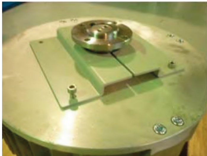
SCREW M8x25 TCEI SS (already on the motor) NUT GROWER D.8 (already on the motor)
